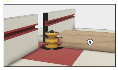
With the rails completed, you can replace the coping bit with the profile cutter. To set the bit height, place one of the coped rails on the router table and adjust the bit until it aligns with the profile in the end of the part.
