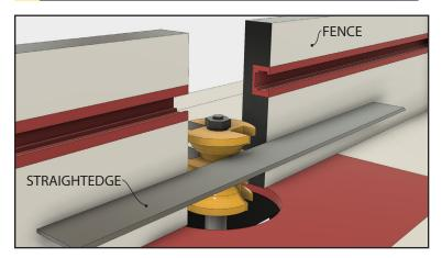
Use a straightedge to set the fence flush with the narrowest part of the profile cutter near the center of the bit and just above the straight cutter. Rotate the bit with your finger until it is perpendicular to the fence. Place the straightedge against the bit and pull the fence forward until it contacts the straightedge. Lock the fence in place.
