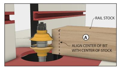
Secure the coping bit in your router table and adjust the height until the center of the bit is aligned with the center of your stock's thickness.
