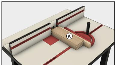
Use a miter gauge with a backer block to cope the ends of your rails. You can route a test piece first and make adjustments to the bit height if necessary. Do not remove the coping bit until you have routed both ends of every rail in your project.
