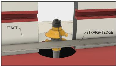
Use a straightedge to set the fence flush with the router bit's bearings. Place the straightedge against the bit and pull the fence forward until it contacts the straightedge. Lock the fence in place.
